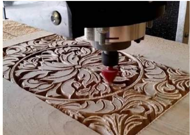
CNC machine carving wood- photo by By WayKen Rapid Manufacturing .
