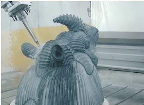
Top- CNC machine carving stone- photo by By WayKen Rapid Manufacturing .
